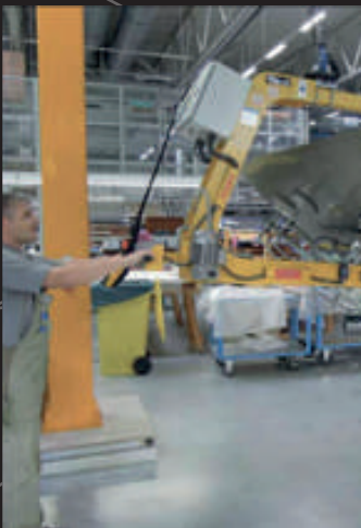
Grippers with possibility of rotatable by 180 degrees and lifting capacity max. 2500 kg
