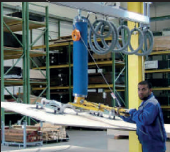
VacuPowerLift VPL Tube lifters for tiltable sheets handling
