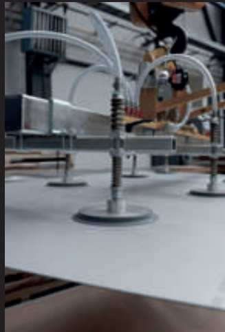
Grippers to horizontal transport of details from 80 to 40,000 kg
