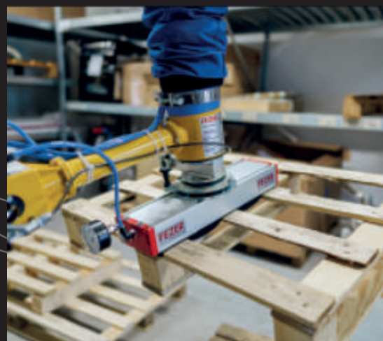
VacuPowerLift VPL Tube lifters with max lifting capacity 200 kg
