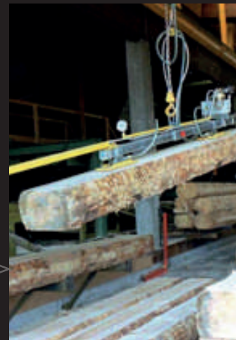
Handling grips load-bearing timber max. 1000 kg
