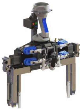
Gripper for picking up of computers from a collection box
