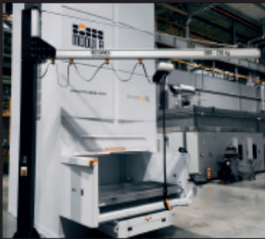
Pillar cranes with aluminium jibs with max. load capacity 1200 kg
