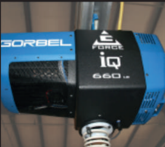
Intelligent assist device ensuring smooth movement
