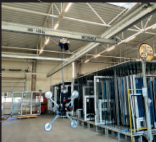
Light aluminum overhead cranes of any size configuration and load capacity up to 1,500 kg
