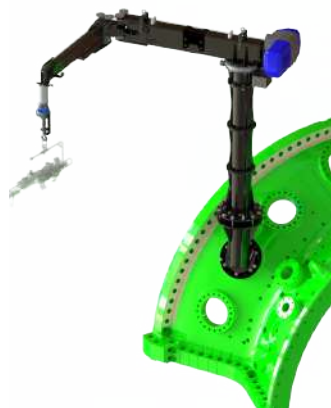
Manipulator with modular mast
