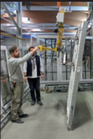
Window grippers of any configuration and load capacity max. 650 kg
